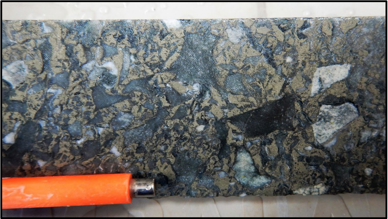
Figure 8: Polymictic volcanic breccia with matrix sulphide replacement. Typical Horseshoe Lights mine sequence stratigraphy (BBDD001 @ 285.1m)
