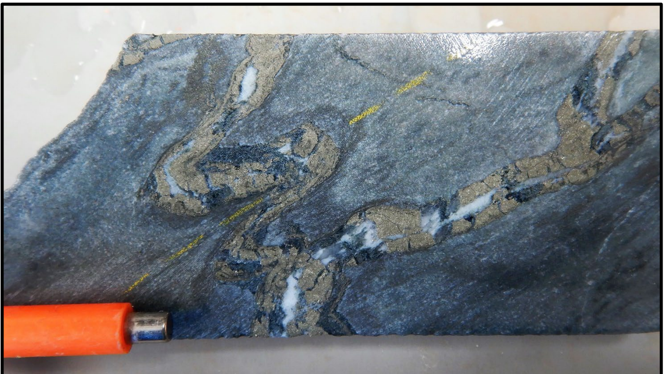
Figure 12: Laminated syn-VMS quartz-pyrite-chlorite veins in sericite altered footwall volcanics, folded in axial planar foliation (BBDD001 @ 271.4m)
