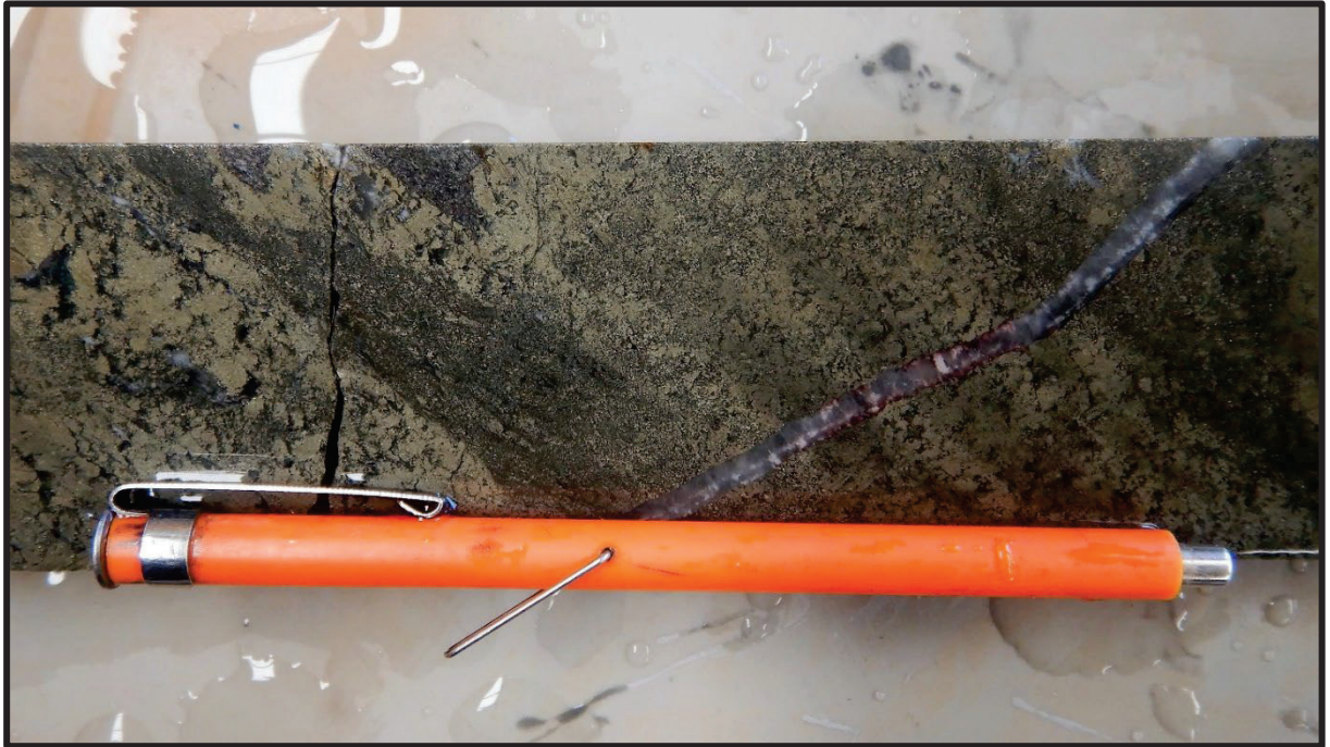
Figure 1 Example banded/laminated massive sulphide (BBRD070 @ 209.2) from within 5.95m zone (BBRD070 203.97 – 209.92m)
