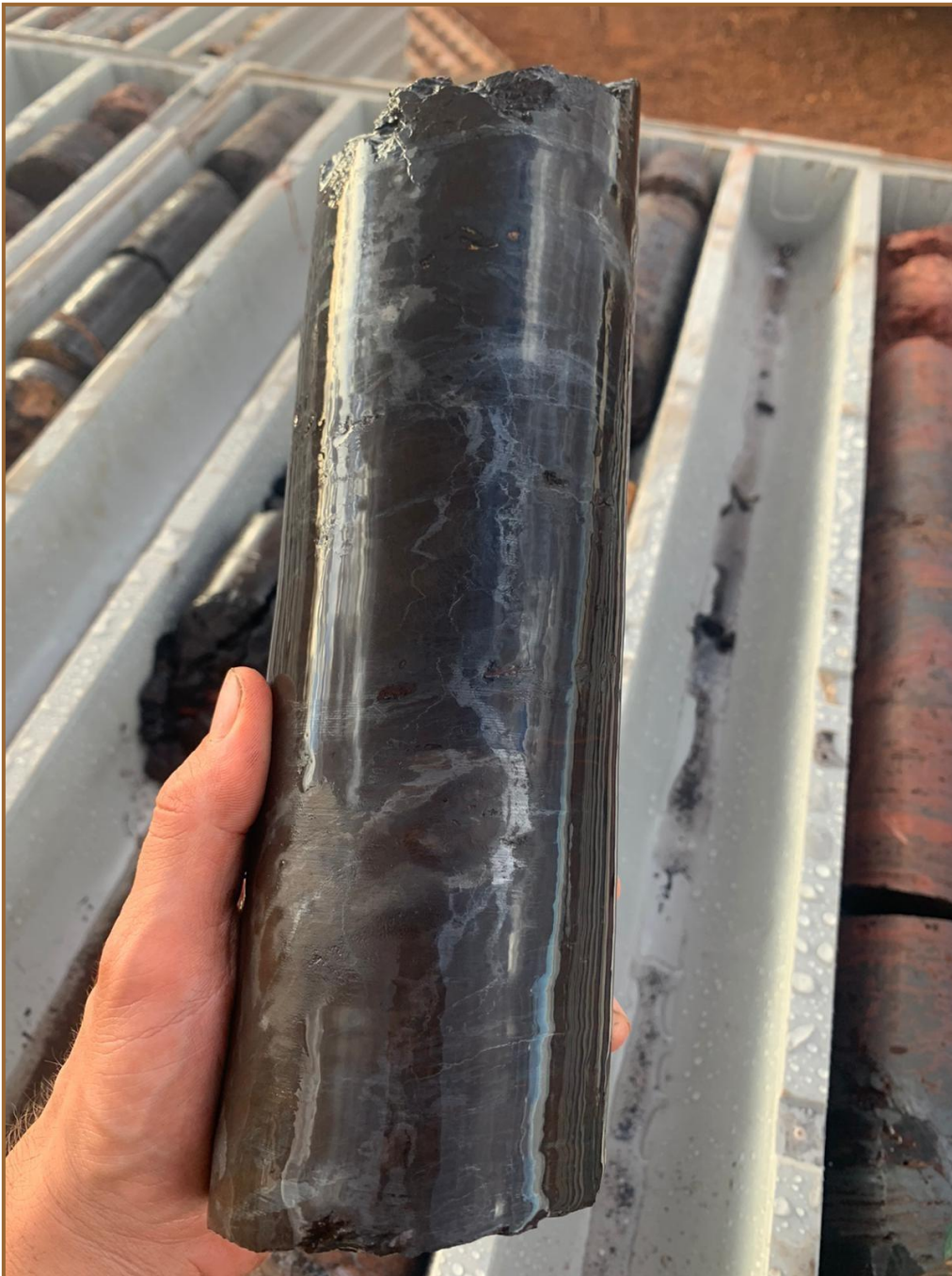
Plate 1 – ~40% Manganese core from BRDD005 (10.2m – 10.4m)
