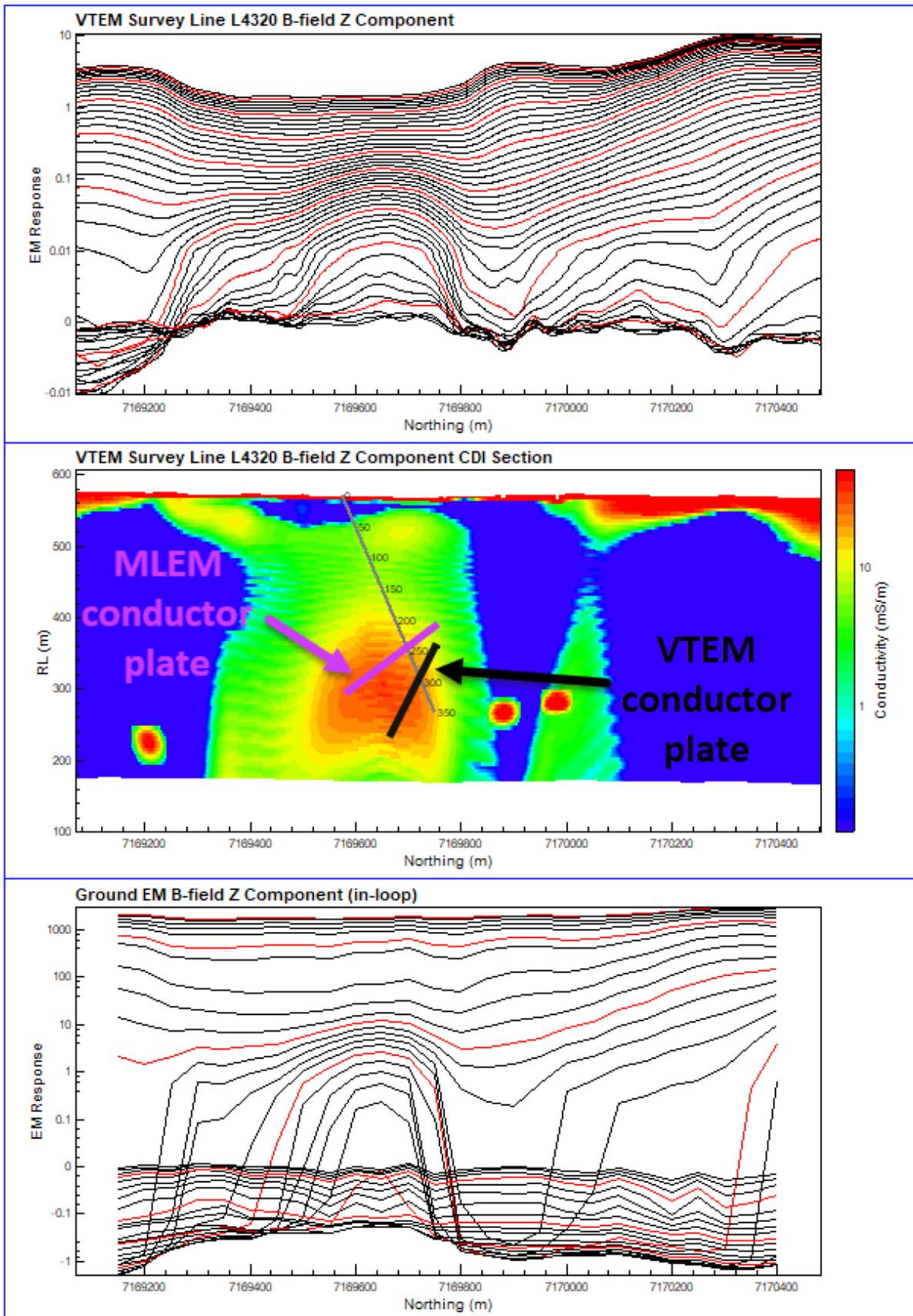
Figure 5 – PH-1 EM target VTEM EM survey decay profile (top), VTEM conductivity cross-section with modelled plates conductor plates used to plan deep RC drilling (middle), and MLEM survey EM profiles (bottom) for survey Line 658900mE, which crosses through recent deep RC drillhole BBRC050.
