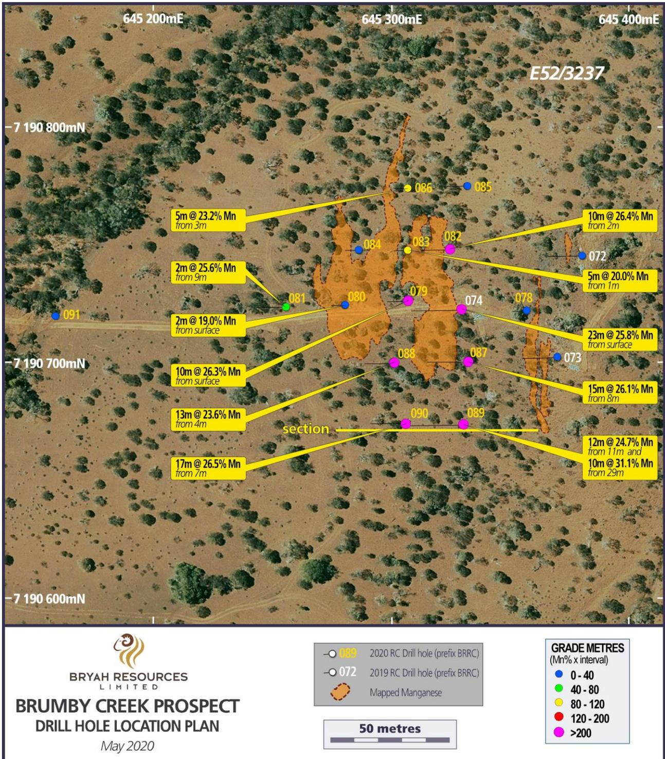
Figure 3 - Brumby Creek Prospect - Drill Hole Location Plan
