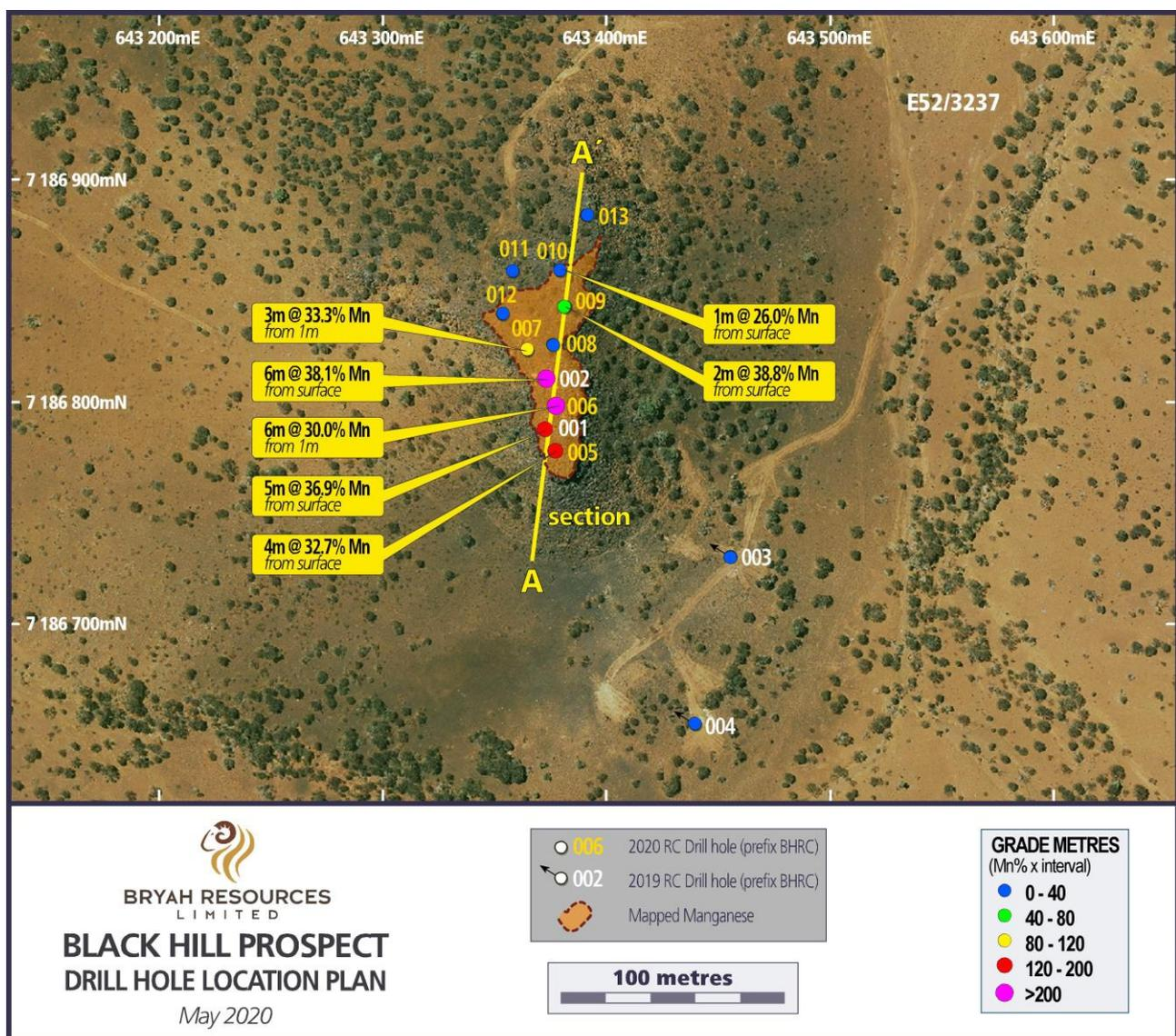
Figure 5 - Black Hill Drill Hole Location Plan
